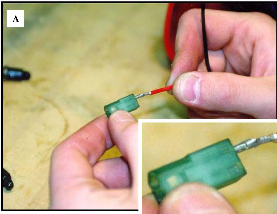
17. Separate the black and red ends of the wire. Guide the red wire into pinhole 1 of a mating connector (rounded on opposite end). Guide the black wire into pinhole 2 of the same mating connector (square on opposite end). **(A)**
