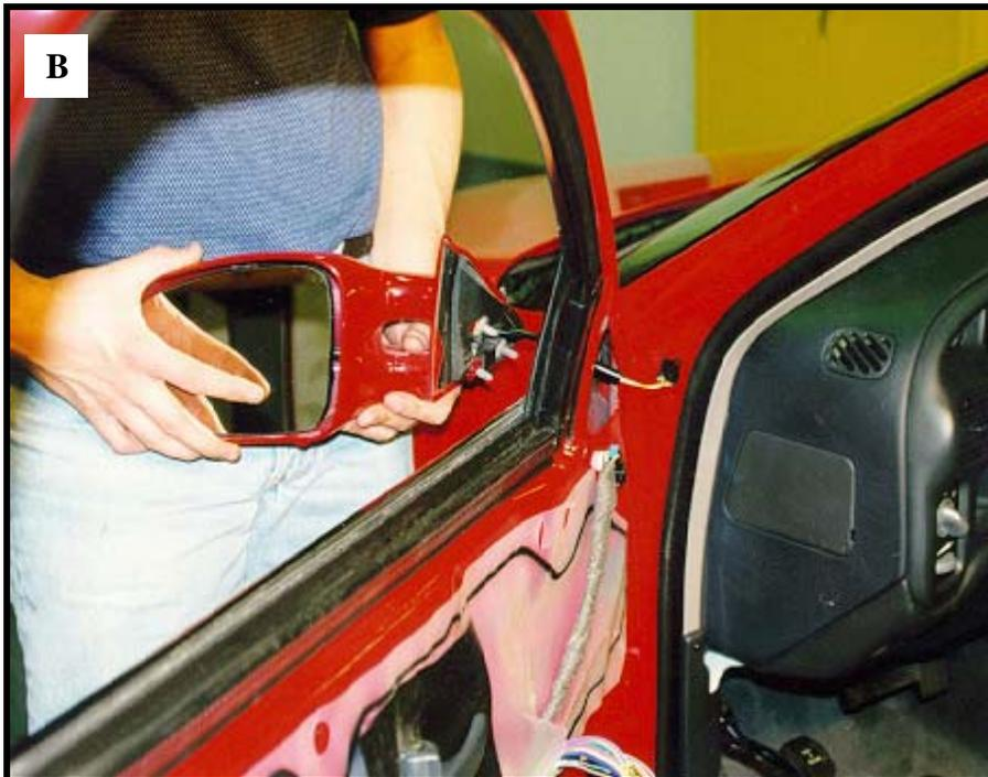
10. Remove the mirror housing from the door. (B)
