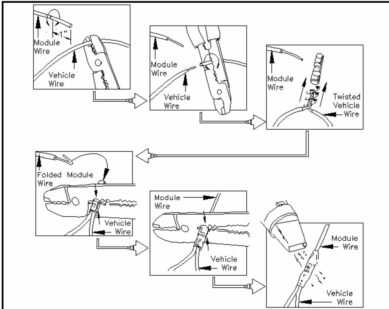
**USE THE DIAGRAM ABOVE TO SPLICE INTO THE TURN INDICATOR WIRES**
