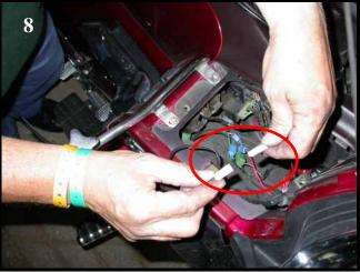
Plug mirror into motorcycle harness. Turn ignition on, test the *Signal*® mirror for functionality.
