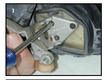
Remove the three screws holding the hinge to the mirror housing. Remove the hinge and remove the rubber boot surrounding the mirror housing.
