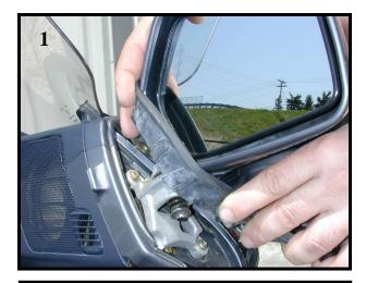
Start on either the left or right side mirror. These instructions start with the right side mirror. Pull back the rubber boot covering the mirror mount.
