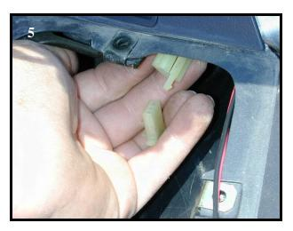
The motorcycle's electrical wiring for turn indicators is located forward of the accessory compartment cavity and behind the front amber turn indicator light. Disconnect the wire connected to the turn indicator light.
