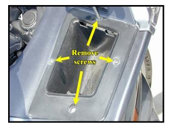
Remove the accessory compartment cover. Remove the four screws on all sides of the accessory compartment. Remove the accessory compartment from the motorcycle fairing and set it aside.
