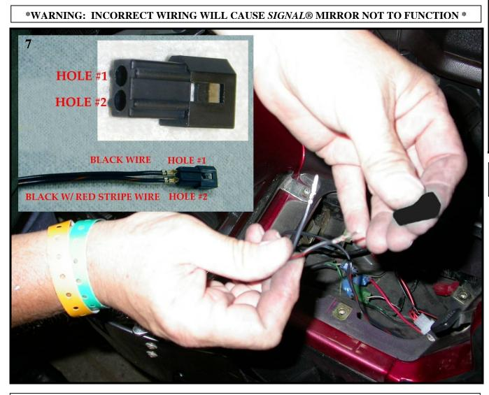
Insert pins into female connector. **NOTE: Insert pin from the black wire into hole #1. Put the pin from black with red stripe into hole #2.**
