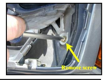
There are three screws holding the mirror housing to the mirror mount. Remove the three screws. Set the mirror housing aside.
