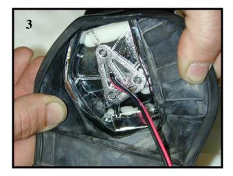
Position the rubber boot over the *Signal*<sup>®</sup> mirror housing.
