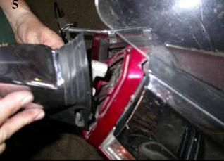
Reinstall Signal<sup>®</sup> mirror onto motorcycle
