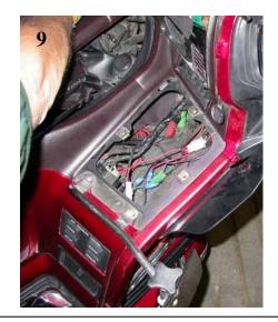
Tuck wiring into fairing. Replace accessory compartment cover, rubber boot, etc. Repeat steps for the other *Signal*® mirror.
