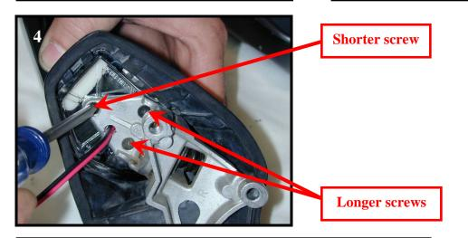
Guide the *Signal*<sup>®</sup> mirror wire harness through the drilled hole in the hinge. Mount the hinge on the *Signal*<sup>®</sup> mirror housing using the original three screws.
