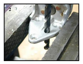
Match the base of the hinge up to the new *Signal*<sup>®</sup> mirror housing. Mark the place on the hinge where the *Signal*<sup>®</sup> mirror wire will go through. Drill a <sup>1</sup>/<sub>4</sub>" hole in the hinge.
