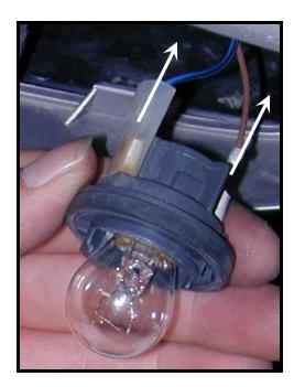
**For bike maintenance purposes:** If you have to remove the mirror from the mirror housing, you will have to use a screwdriver and remove the screw from the front turn indicator lens. Disengage the lens and remove the light bulb as shown. Disconnect the *Signal*<sup>®</sup> mirror wire harness from the light bulb and the motorcycle's side turn indicator via the Y-connector. Remove the mirror from the mirror housing.
