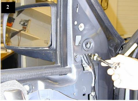
1. Open the driver side door and lower the window. Remove screw (A) using a slotted screwdriver. Using a 7mm socket, removed screw (B & C). Pry open the cover (D), for the control panel and the door handle, using a pry bar. Disconnect connectors on control panel. Pry open cover behind grab bar and remove the two screws using a torx wrench #27 (E). Pry around door panel, disconnect any remaining wire connectors, and remove door panel.
