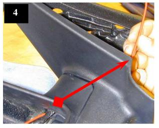
4. Remove foam covering from housing sail. Insert the open end of the supplied *Signal*® mirror wire harness thru housing (following OE wires). Pull the *Signal*® mirror wire harness thru leaving about 5" of slack inside housing. Following OE wires, continue routing the *Signal*® mirror wire harness thru sail cover. Replace sail cover.
