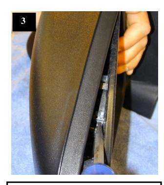
3. Using sturdy gloves, press down on the inboard side of the mirror to pivot it fully outward. Using a large flathead screwdriver, reach in between the motor actuator and the motor mount. Slowly twist and pry until the mirror disengage from the mirror housing. **If heated,** disconnect heater terminals. Remove mirror from mirror housing.
