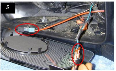
5. Connect the *Signal*® mirror mating connector to the *Signal*® mirror wire harness. Connect the factory heater wires to the heater terminals on the *Signal*® mirror. Align the anti-rotation groove with the prong on the motor actuator. Carefully tuck the anti-vibration tabs inside mirror housing. Centering the snap ring on the motor actuator and slowly push down on the glass until the mirror snap into position. Push down on all sides to ensure proper engagement and functionality.
