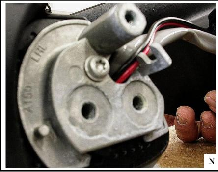
Continue routing the *Signal*<sup>®</sup> mirror wire harness thru the sail and plastic insulation (M). **CAUTION:** When replacing the sail, make sure to position all wire harnesses as shown on (N). Not doing so could result in wiring harnesses being crushed by the sail, when re-assembling, causing shortage in the long run. Re-assemble the sail back onto the mirror housing. Replace the plastic insulation onto the housing sail.
