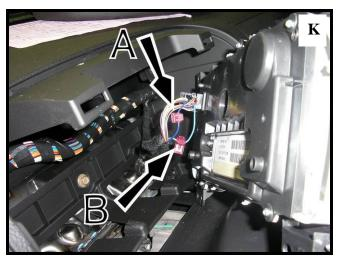
The vehicle's electrical wirings are located on the driver side, behind the instrument panel. To gain access to the wiring location, first remove the driver side lower dash. Second, remove the instrument panel trim cover by pulling straight toward the driver seat (I). Lastly, remove the (4) 7mm screws around the instrument panel (J). Route the BLACK w/ RED TRACE wire on both *Signal*<sup>®</sup> mirror wire harnesses to the wiring location behind the instrument panel.
