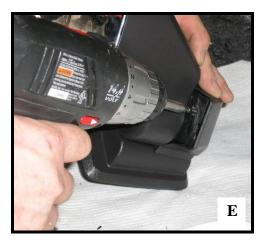
Push down on the lower edge of glass until mirror pivots fully outward (**A**). Using a small pry bar, carefully pry the mirror up toward the top until mirror pops loose (**B**). **If heated**, disconnect heater wires from heater terminals and remove mirror (**C**). Unscrew and release the (4) #15 torx screws which attach the mirror housing to housing arm (**D**). Remove (1) #15 torx screw located on the lower half of the mount (**E**).
